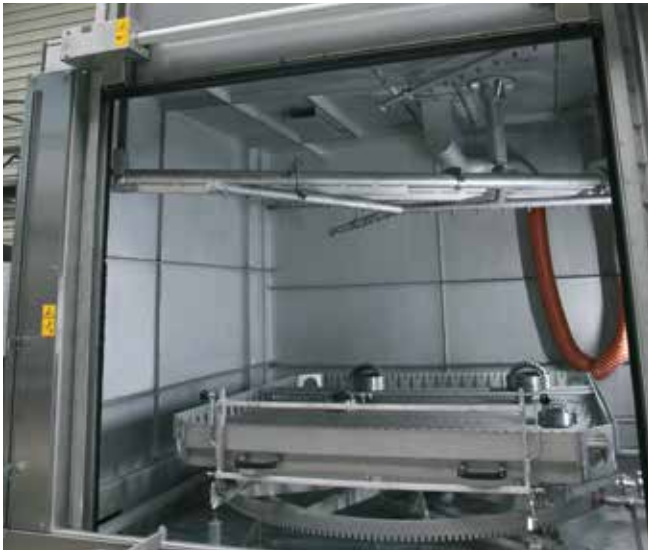
Version Lowerable nozzle frame for different washing heights
