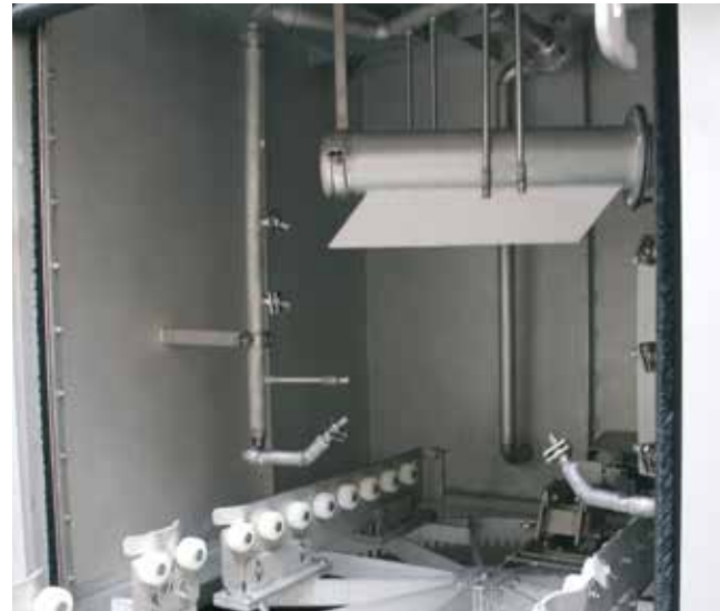
Version Drying nozzle adapted to the component
