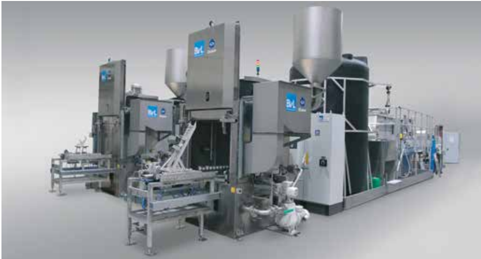
Version Ocean RW with central supply to lower operating costs and decentralize maintenance and service points
