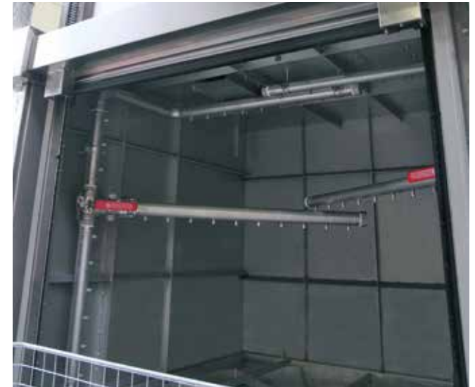
Version Bayonet connection for adjusting the nozzle frame to two different heights
