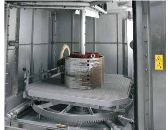
Version Center lance to thoroughly clean internal components
