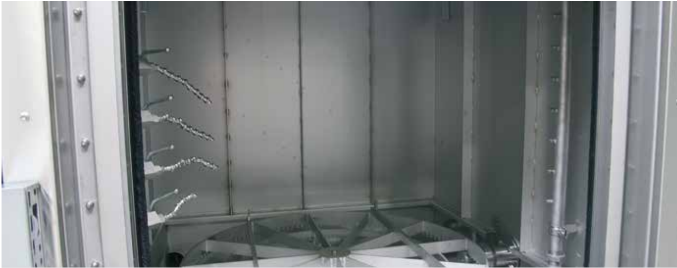
Version Nozzle system individually adapted to the components
