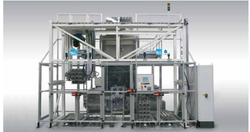
Version Ocean RW with loading portal for unmanned operation
