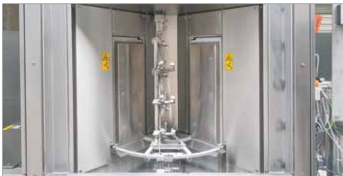
View of the loading/unloading zone: here with a customer-specific mount for parts
