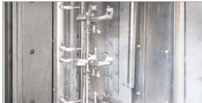
View of the drying zone: Drying with a rotating nozzle system and high-performance side channel blower
